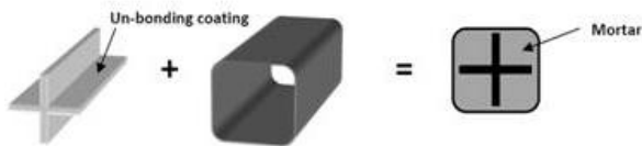
Figure 1 – Typical Buckling-restrained brace configuration. A steel core plus a steel restraining tube and mortar, make up the BRB cross section.
