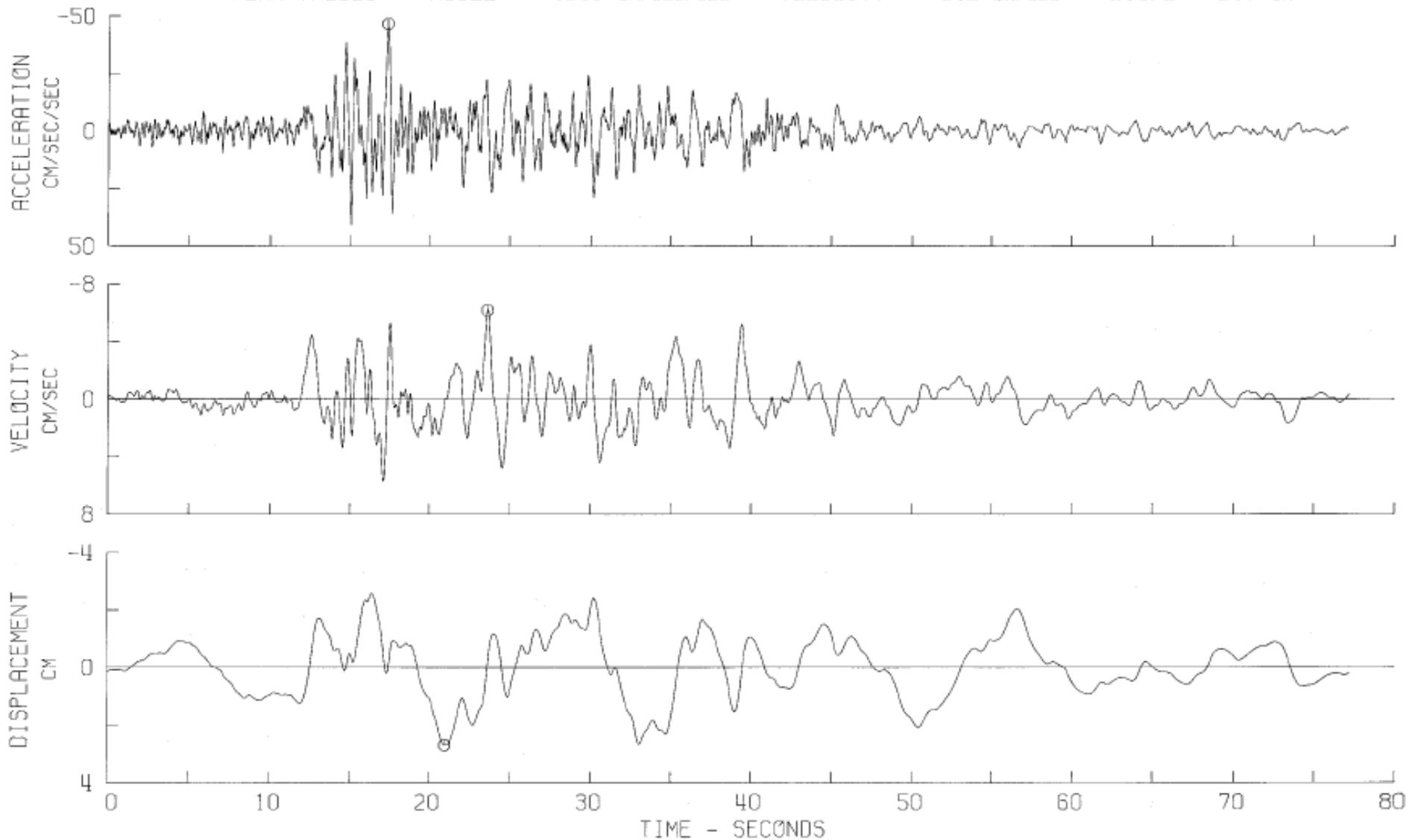
For a given earthquake ground excitation record (time history), ground motion parameters describe the earthquake shaking characteristics of importance (e.g., amplitude, frequency content, and duration).
