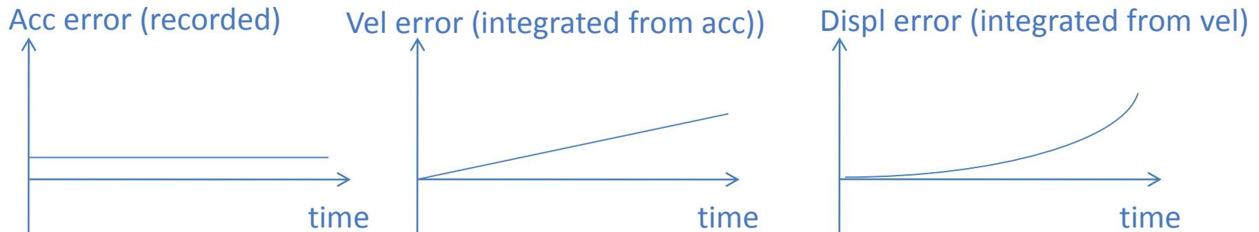
For instance, if the entire recorded acceleration time history is erroneously offset by 0.0001 m/sec and the record duration is 100 seconds, this error will translate into a velocity of  $.0001 \times 100 = .01$  m/sec at the end of the record, and a permanent displacement of 0.5 m (also at the end of the record).
